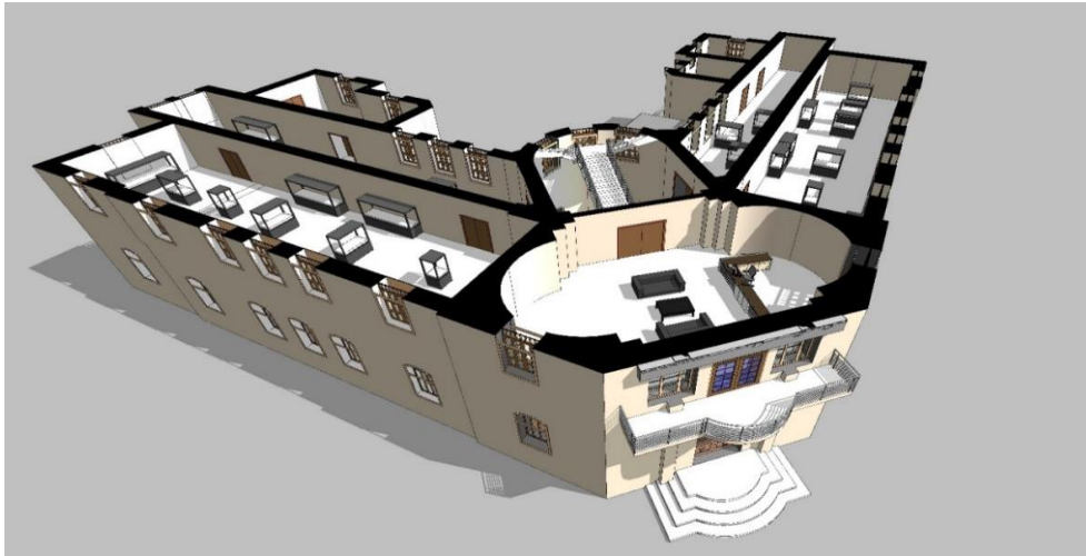
Figure 1. 3d perspective of Museum Modeled using Revit Showing Furniture and cabinet's distribution
