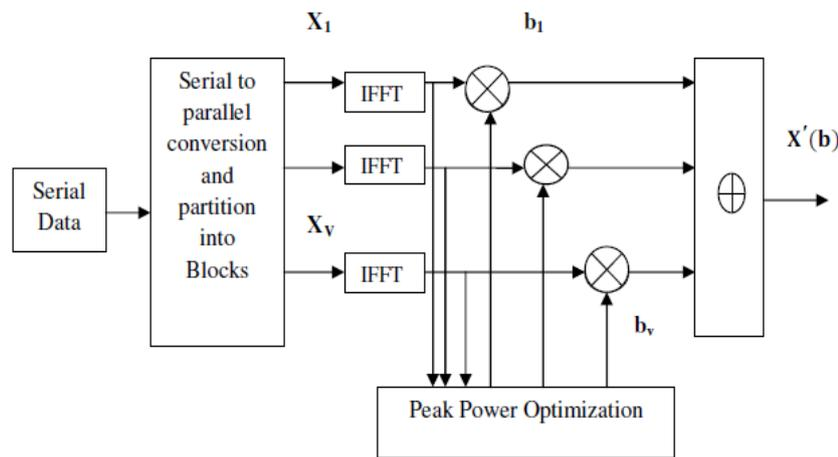
Figure 3. PTS Block Diagram
