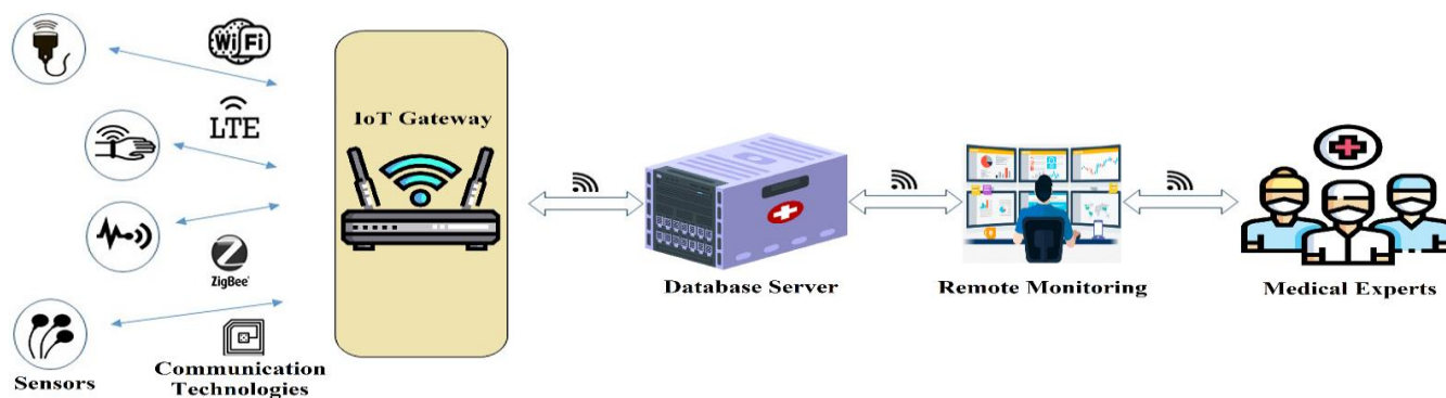
Figure 1. Common Architecture of Medical IoT
