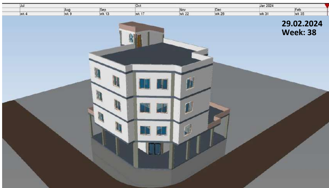
Figure 26: masonry work for the 3 rd floor completed
