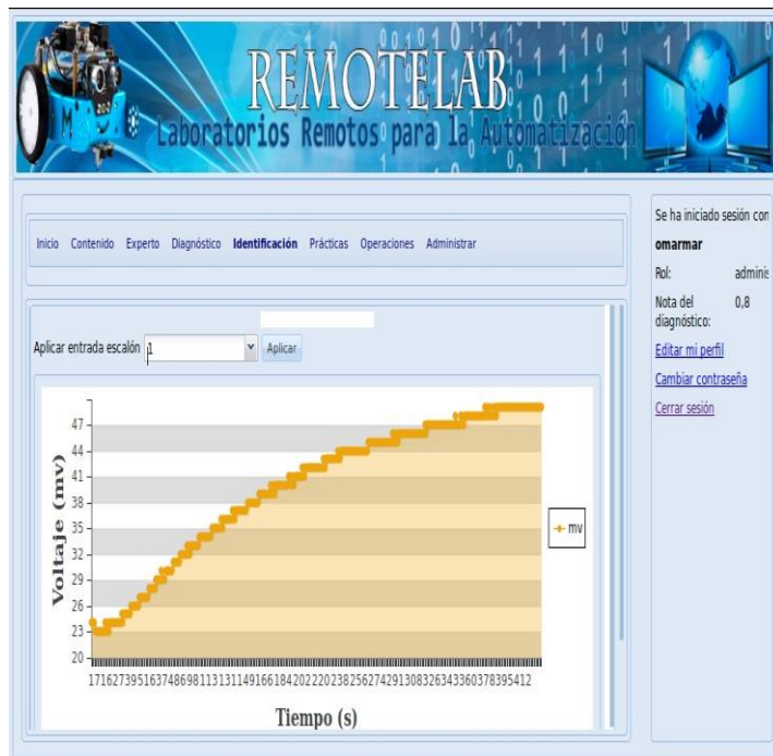
Figure 6. System identification interface from the reaction curve.
