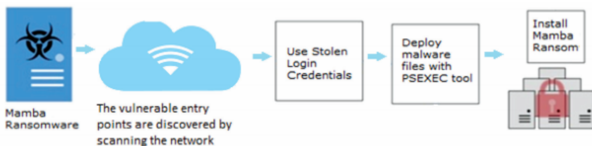
Figure 1 – An Illustration of How Ransomware Attacks ( Source: [12])
