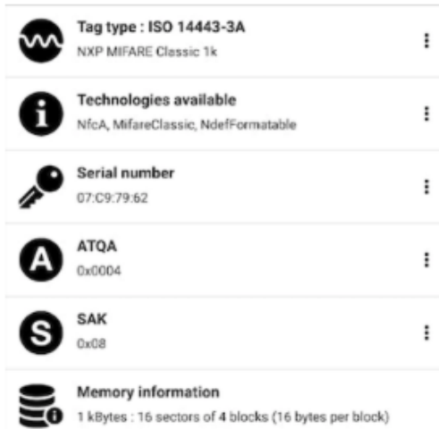
Figure 11: Data extracted using a mobile NFC app (card)
