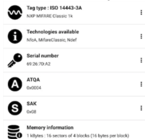
Figure 12: Data extracted using mobile NFC app (Token)
