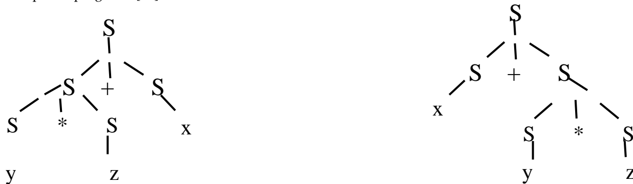
Two parse trees that describe CFGs that generate the string "x + y * z". Source: Context-free grammar
