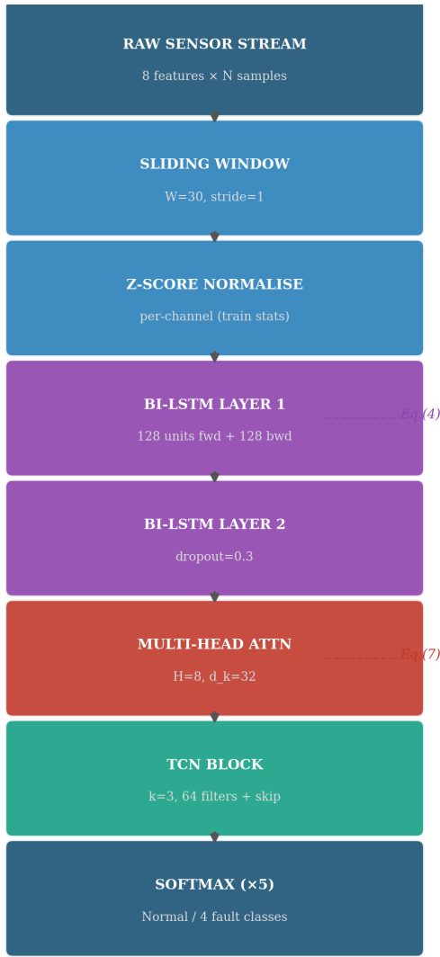
Figure 2. TA-FaultNet block diagram. Raw sensor streams are segmented into W=30 windows, encoded by two bidirectional LSTM layers, attended by H=8 parallel self-attention heads, compressed by a temporal convolutional block, and classified by a five-class softmax.
