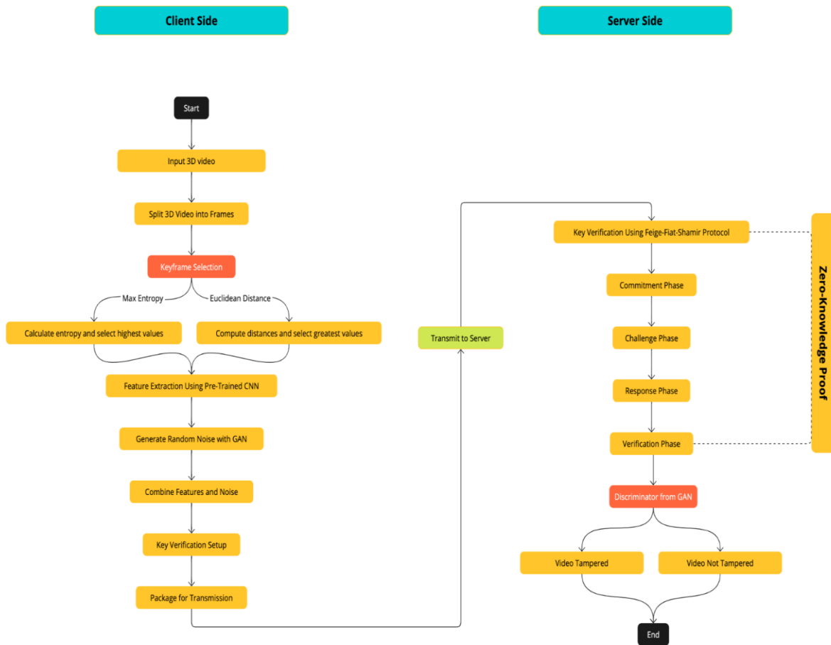
Figure 1. Proposed System Block Diagram.
