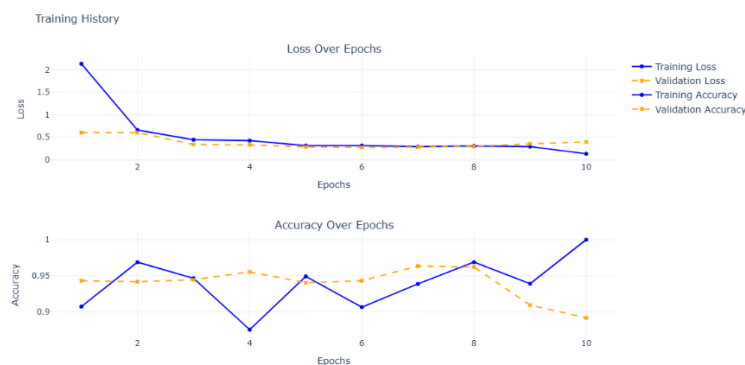
Figure 10. Training and validation loss and accuracy results for VGG19 model
