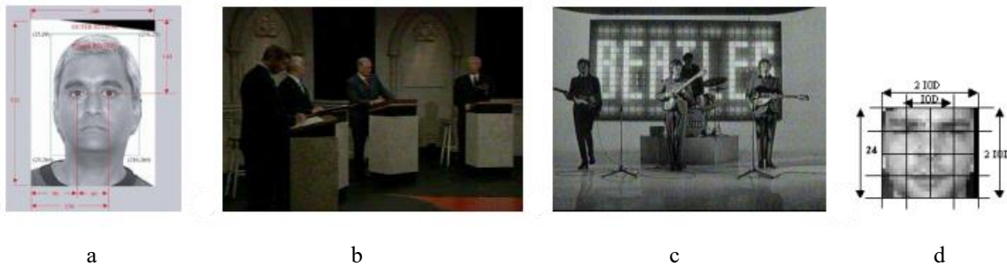
Figure 1. Face image utilized for face recognition in documents (a), face images captured from video (b, c), and a face model appropriate for video-based face analysis (d).
