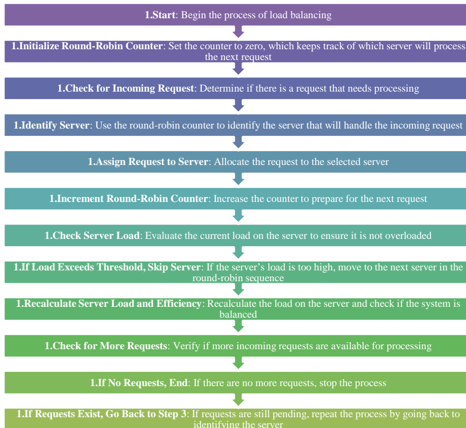
Figure 1. Round-Robin Load Balancing Algorithm in Web Systems.
