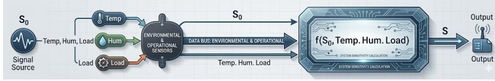
Figure 3. Equivalent schematic model of energy metering system
