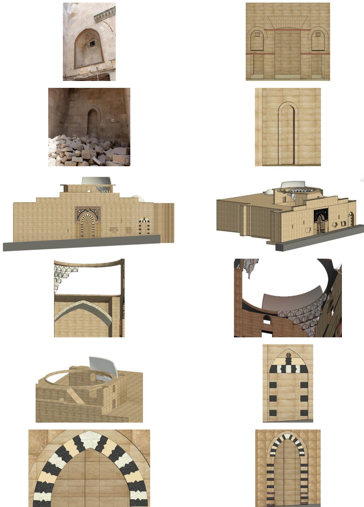
LOD350 and LOD400 modeling outputs: openings, mihrab, current-state geometry, and ablaq-stone details.
