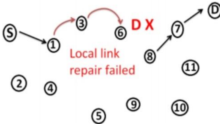
Figure 2: failure of the local repair process due to distance from the target
