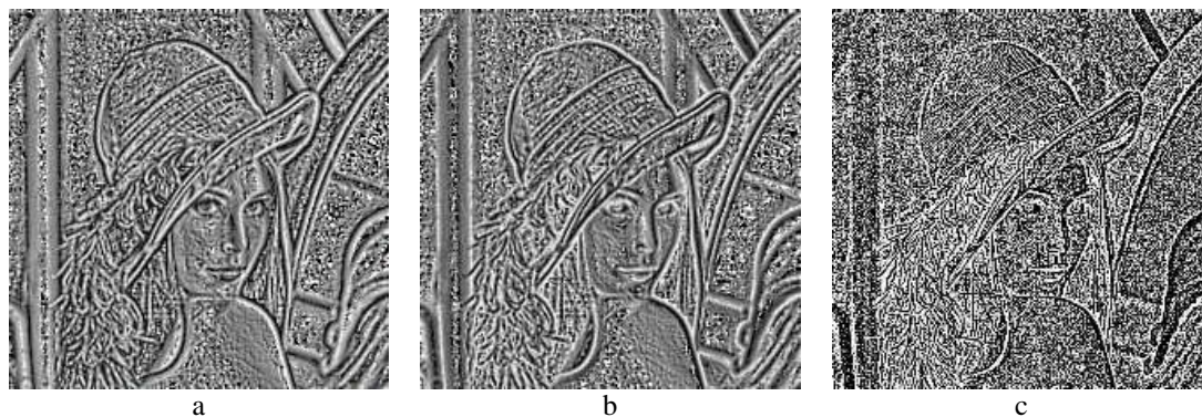
Figure. 3 Lena Image in Neutrosophic Domain (a) True Image (b) False Image (c) Indeterminate Image
