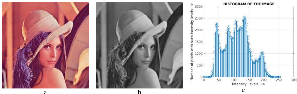
Figure 2: (a) True Lena Image, (b) Gray Scale Lena Image, (c) Histogram of Lena Image (b)
