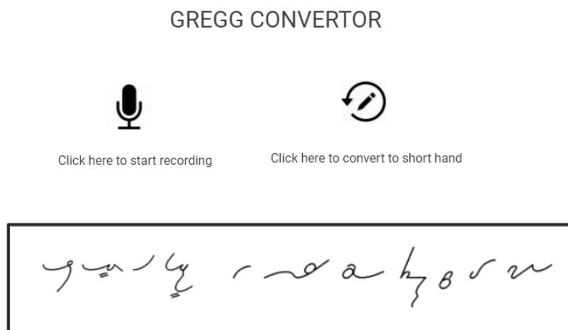
Figure 3: The diagram shows user interface of our proposed Gregg converter. The record button is clicked to recorder the speech. Once recorded, the converter button is enabled and when clicked, displays the shorthand in the text box as shown above.
